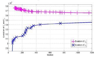
Fig. 5. The variation of  $\xi_1$  and  $\xi_2$  at -5 dB using M-HSD algorithm, with  $\gamma = 1$ , N1 = 30, and N2 = 30. Each mark on the curves indicates a modification of  $\xi_1$  and  $\xi_2$ .
