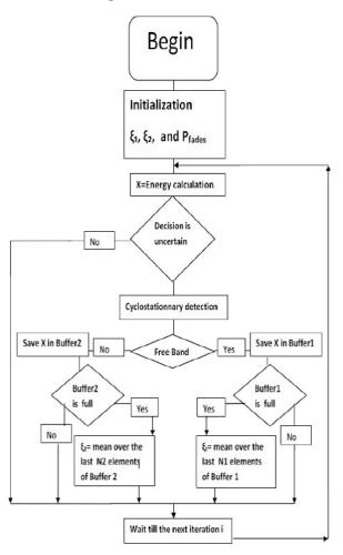
Fig. 4. Modified version of the HSD algorithm (M-HSD)
