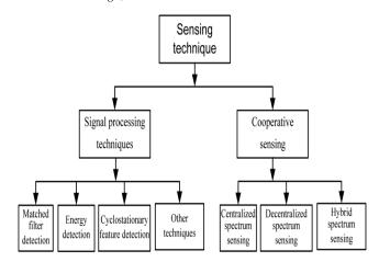
Fig. 1. Various Spectrum Sensing techniques.
